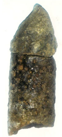
Used blow pipe in crucible furnace
